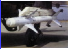
A PL-9 missile fitted to a J-7 ( MiG-21 'Fishbed') aircraft ( CATIC )
