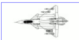
Documents obtained by JDW suggest that the J-10 will feature 11 hard points
